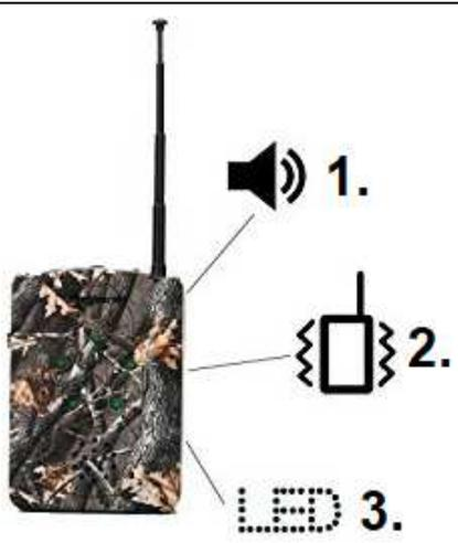
The diagram shows a rectangular receiver device with a camouflage pattern. Three callout lines point to specific features: '1.' points to a speaker icon, '2.' points to a vibration icon (a square with a vertical line and wavy lines), and 'LED 3.' points to a small LED light on the front of the device.
